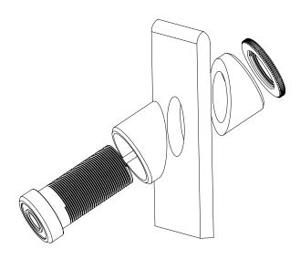
Installing IRIS-S435 with Angle Wedges
