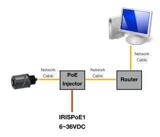
As mentioned previously, the camera as default is set to obtain its IP address automatically via DHCP. This means that once connected, your router will detect the device and assign it an IP address within its designated range (refer to the documentation for your router for further details). You must also ensure the network adapter for your computer is set to obtain its address via DHCP.
