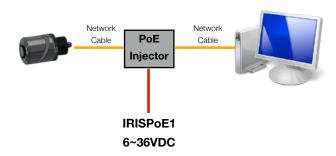
Use a standard 568B ethernet CAT5 cable to hook your computer up to the PoE injector, and then another 568B cable to hook the camera up to the injector.
